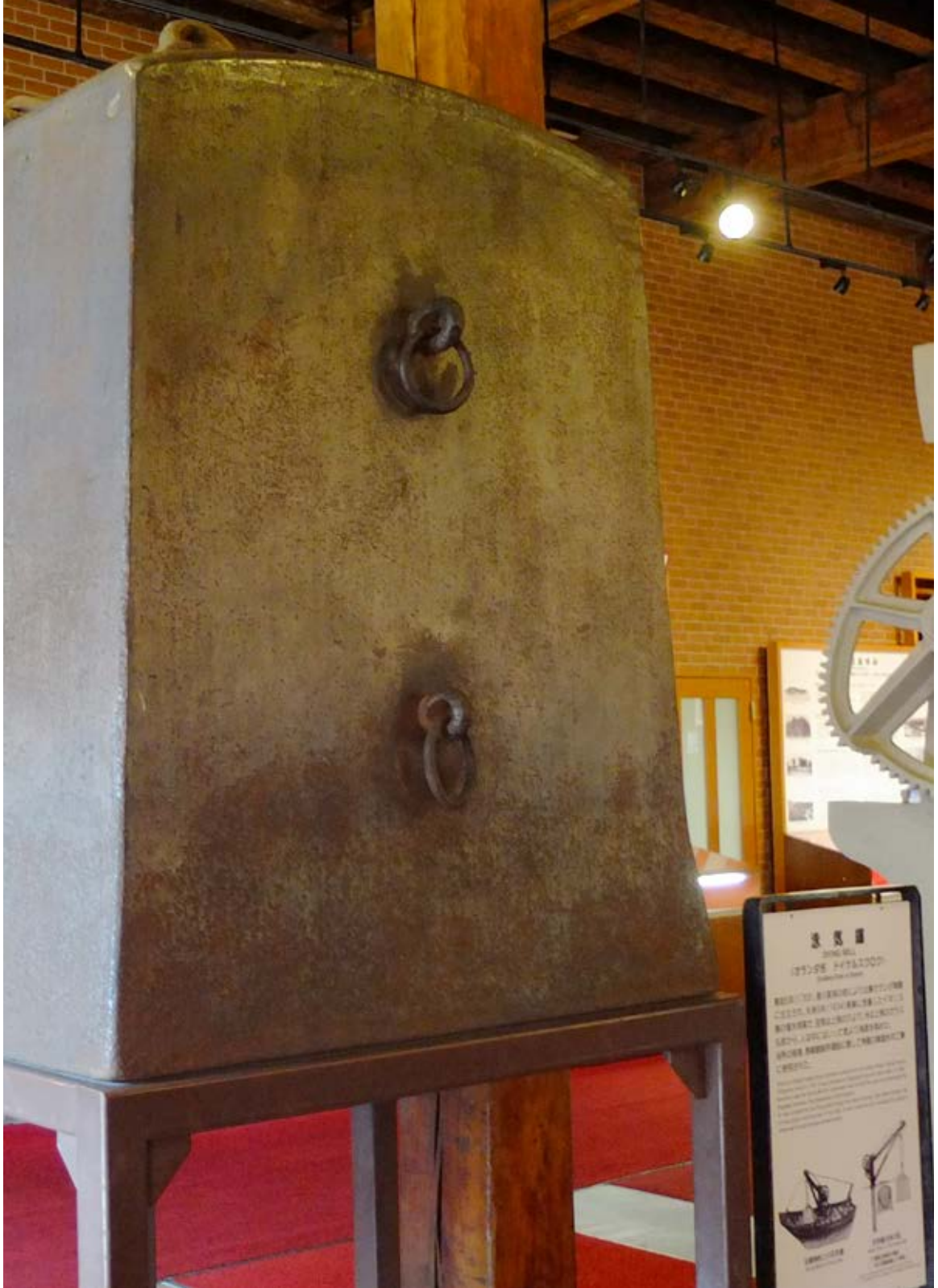
Figure 36 The original diving bell used by the Dutch marine officers to built the wharf near the steam engineering factory in Nagasaki, on display in the Mitsubishi Museum in Nagasaki (Derksen, 2013).
